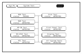
14 Install a formatted disk that is not write protected into the disk drive. If option 020 is installed, connect an RS-232C loopback connector onto the RS-232C port. Run the remaining System Tests in the same manner.
